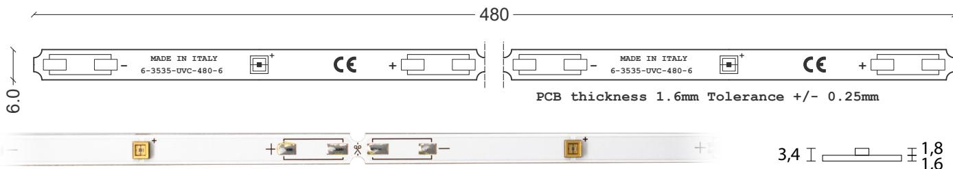
ATTENTION the module can be sectioned but with a special blade
