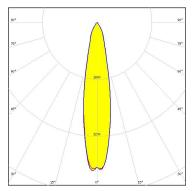
Dimensions: 70.0 mm x 70.0 mm Height: 42.00 mm ~15° spot beam
