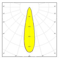
Dimensions: 70.0 mm x 70.0 mm Height: 42.00 mm ~24° medium beam
