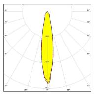
Dimensions: 49.9 mm x 49.9 mm Height: 25.00 mm ~15° spot beam
