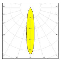
Dimensions: 49.9 mm x 49.9 mm Height: 25.00 mm ~24° medium beam
